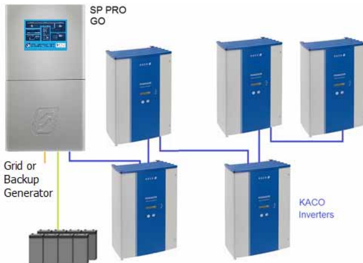
RS485 wired communications links between SP PRO GO and KACO inverters
