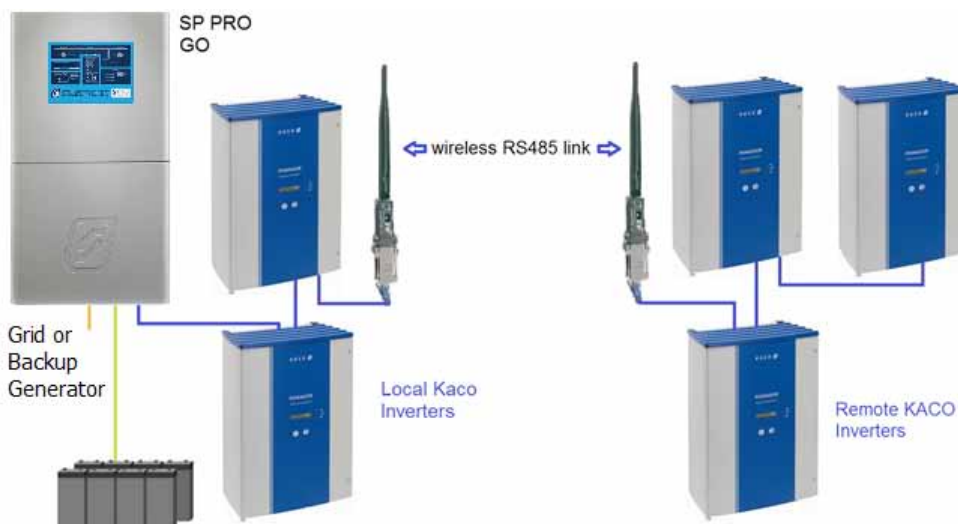
RS485 wired AND wireless communications links between SP PRO GO and KACO inverters
